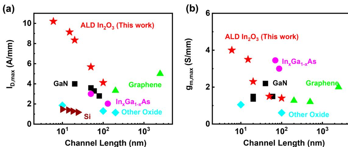
**Figure 4.** Benchmarking of ALD  $\text{In}_2\text{O}_3$  with other semiconductor materials. Comparison of (a)  $I_{D,\text{max}}$  and (b)  $g_{m,\text{max}}$  versus channel length characteristics with other high-performance semiconductor materials and graphene. Transistors with ALD  $\text{In}_2\text{O}_3$  demonstrate the largest  $I_D$  and  $g_m$  compared to all known semiconductors with a planar structure due to the high carrier density and high velocity.
