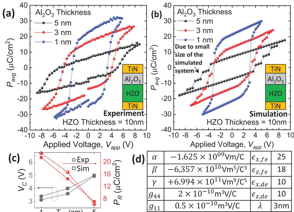
FIG. 1. (a) Measured and (b) simulated *P*<sub>avg</sub>-*V*<sub>app</sub> characteristics of FE-DE stacks for different *T*<sub>DE</sub>. (c) Average *V*<sub>C</sub> (*V*<sub>app</sub> at *P*<sub>avg</sub> = 0) and *P*<sub>R</sub> (*P*<sub>avg</sub> at *V*<sub>app</sub> = 0) for different *T*<sub>DE</sub>. (d) Table showing the simulation parameters.
