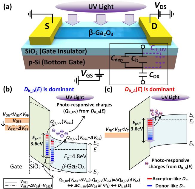
**Fig. 2.** (a) Schematic view of the measurement setup under a photonic state with the sub-bandgap UV light including the equivalent circuit model as the inset. (b) and (c) Energy band diagrams for the concept of simultaneous extractions of both  $D_{it\_D}(E)$  and  $D_{it\_A}(E)$ .
