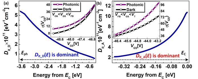
**Fig. 4.** Energy distribution of extracted  $D_{it}$  [(a):  $D_{it\_D}(E)$  and (b):  $D_{it\_A}(E)$ ] via photo-responsive I-V characteristics with sub-bandgap UV light. The inset shows the extracted  $\eta(V_{GS})$ .
