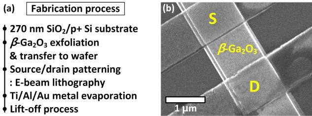
**Fig. 1.** (a) Process flow for device fabrication of the exfoliated  $\beta$ -Ga<sub>2</sub>O<sub>3</sub> nano-membrane FETs with the bottom-gate structure. (b) SEM image of the fabricated device.
