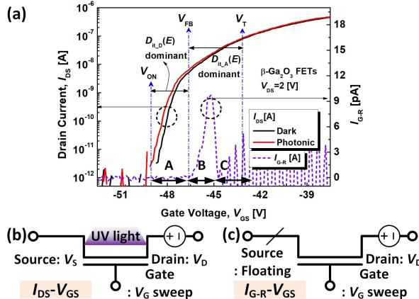
**Fig. 3.** (a) Measured  $I_{DS}$ - $V_{GS}$  characteristics under dark (black line) and photonic (red line) states. The  $I_{G-R}$  (dash line) was measured with the source terminal floating. Measurement setup for (b)  $I_{DS}$ - $V_{GS}$  with UV light and (c)  $I_{G-R}$ .
