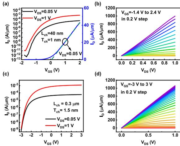
Fig. 4. (a)  $I_D$ - $V_{GS}$  and (b)  $I_D$ - $V_{DS}$  characteristics of an  $\text{In}_2\text{O}_3$  transistor with  $L_{ch}$  of 40 nm and  $T_{ch}$  of 1 nm. (c)  $I_D$ - $V_{GS}$  and (d)  $I_D$ - $V_{DS}$  characteristics of an  $\text{In}_2\text{O}_3$  transistor with  $L_{ch}$  of 0.3  $\mu\text{m}$  and  $T_{ch}$  of 1.5 nm.
