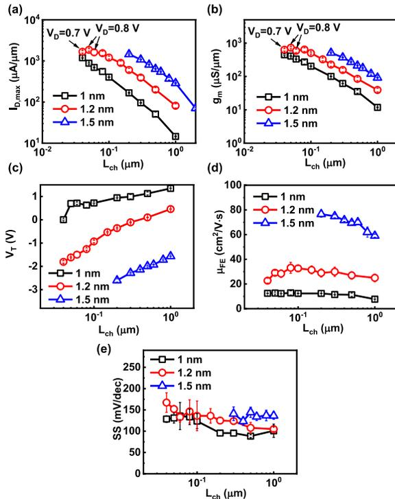
Fig. 5. (a)  $I_{D,max}$ , (b)  $g_m$ , (c)  $V_T$ , (d)  $\mu_{FE}$ , and (e) SS scaling metrics of  $\text{In}_2\text{O}_3$  transistors with  $L_{ch}$  from 1  $\mu\text{m}$  to 40 nm and  $T_{ch}$  from 1 nm to 1.5 nm.  $I_{D,max}$  and  $g_m$  are extracted at  $V_{DS} = 1 \text{ V}$  unless otherwise specified. Each data point represents the average of at least 5 devices.
