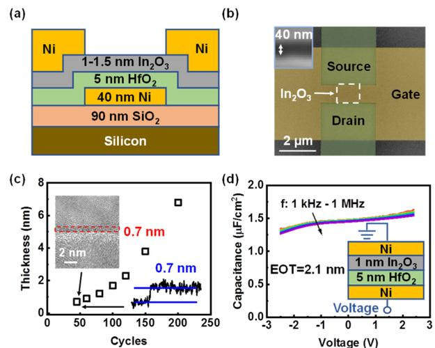
**Fig. 1.** (a) Schematic diagram of an  $\text{In}_2\text{O}_3$  transistor with 5 nm  $\text{HfO}_2$  as gate dielectric. (b) SEM image of a fabricated  $\text{In}_2\text{O}_3$  transistor. (c)  $\text{In}_2\text{O}_3$  thickness versus ALD cycles, showing a nucleation delay process. (d) C-V measurement of the gate stack from 1 kHz to 1 MHz. Smaller capacitance at negative gate bias is due to the depletion of semiconducting  $\text{In}_2\text{O}_3$  channel.
