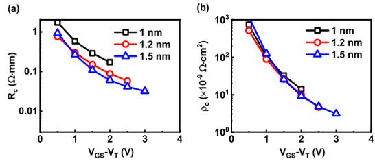
Fig. 6. (a)  $R_C$  versus  $V_{GS} - V_T$  extracted by TLM method for  $\text{In}_2\text{O}_3$  transistors with  $T_{ch}$  from 1 nm to 1.5 nm. (b)  $\rho_C$  versus  $V_{GS} - V_T$  extracted by TLM method for  $\text{In}_2\text{O}_3$  transistors with  $T_{ch}$  from 1 nm to 1.5 nm.
