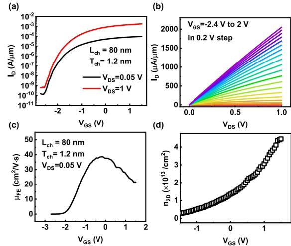
Fig. 3. (a)  $I_D$ - $V_{GS}$  and (b)  $I_D$ - $V_{DS}$  characteristics of an  $\text{In}_2\text{O}_3$  transistor with  $L_{ch}$  of 80 nm and  $T_{ch}$  of 1.2 nm. (c)  $\mu_{FE}$  versus  $V_{GS}$  characteristics extracted at  $V_{DS} = 0.05$  V. (d) Channel mobile carrier density versus  $V_{GS}$  calculated from  $I_D$  and  $\mu_{FE}$ .
