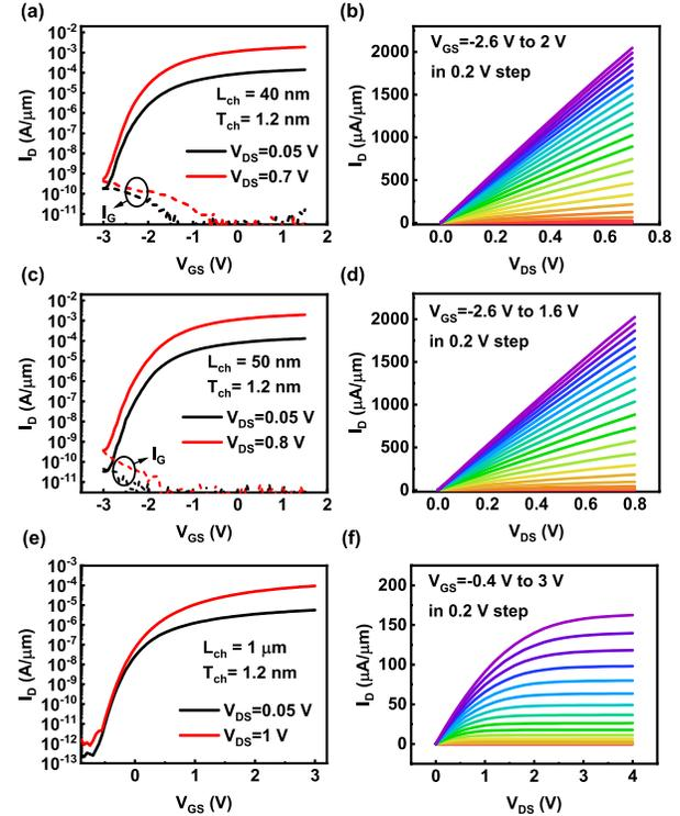
Fig. 2.  $I_D$ - $V_{GS}$  and  $I_D$ - $V_{DS}$  characteristics of  $\text{In}_2\text{O}_3$  transistors with  $L_{ch}$  of (a, b) 40 nm, (c, d) 50 nm, and (e, f) 1  $\mu\text{m}$  and  $T_{ch}$  of 1.2 nm.
