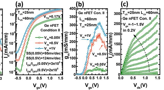
Fig. 9 (a) I<sub>d</sub>-V<sub>gs</sub> curves of a 60 nm L<sub>ch</sub> nFETs in condition II. A low SS of 95 mV/dec is obtained. (b) The g<sub>m</sub> vs. V<sub>gs</sub> relationship of the same device in (a). (c) Output curves of the same device in (a).
