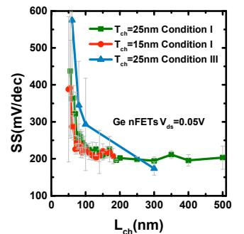
Fig. 13 SS scaling metrics of nFETs with T<sub>ch</sub> of 15/25 nm in condition I and T<sub>ch</sub> of 25 nm in condition III at V<sub>ds</sub> of 0.05 V.
