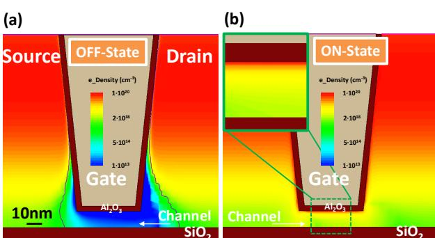
**Fig. 25** (a) OFF-state simulation result of electron distribution of a 50nm  $L_{ch}$  recessed channel nFET by TCAD. The black lines mark the boundary of the depletion region. (b) ON-state simulation result of electron density of the device in (a). Inserted figure shows the enlarged channel area.
