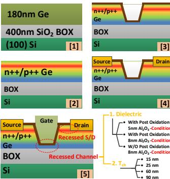
Fig. 2 Device cross sections at different recess depths and S/D MOSFETs. Experiment splits of gate dielectric and T<sub>ch</sub> are listed.
