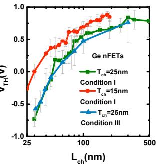
Fig. 10 V<sub>TH</sub> scaling metrics of nFETs with T<sub>ch</sub> of 15/25 nm in condition I and T<sub>ch</sub> of 25 nm in condition III.
