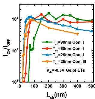
**Fig. 22**  $I_{ON}/I_{OFF}$  ratio scaling metrics of pFETs with  $T_{ch}$  of 25/60/90 nm in *condition I* and  $T_{ch}$  of 25 nm in *condition III* at  $V_{ds}$  of -0.5 V.
