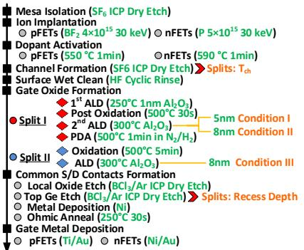
Fig. 1 Fabrication process flow of the Ge MOSFETs. Different recess depths / T<sub>ch</sub> / gate dielectric stacks are studied.
