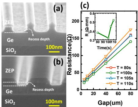
Fig. 4 (a-b) Testing recessed S/D structures with different recess depths. (c) TLM results of recessed contacts on n-Ge with different recess depths (etching time). The inserted figure shows the dependence of R<sub>c</sub> on the etching time. (d) Best TLM results on n and p type contacts.
