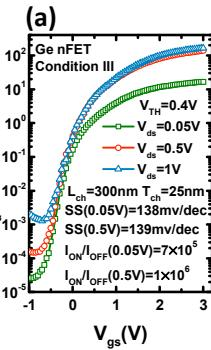
Fig. 8 I<sub>d</sub>-V<sub>gs</sub> curves of a 300 nm L<sub>ch</sub> nFET in condition III with a record high I<sub>ON</sub>/I<sub>OFF</sub>. (b) The g<sub>m</sub>-V<sub>gs</sub> curves of the device in (a).
