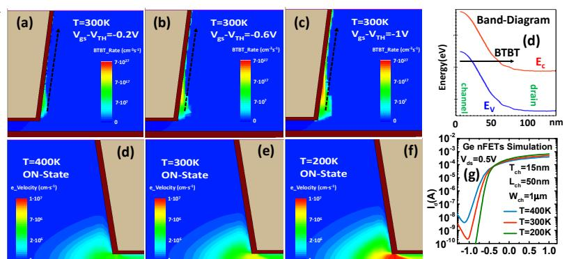
**Fig. 26** (a-c) OFF-state BTBT generation rate ( $\text{cm}^{-3}\text{s}^{-1}$ ) contours of the device in Fig. 25 with  $V_{gs} - V_{TH} = -0.2$ , -0.6 and -1 V at 300 K. (d) Simulated band-Structure along the tunneling path marked by the dashed arrow in (c). (d-f) ON-state electron velocity ( $\text{cm}\cdot\text{s}^{-1}$ ) contours of the same device at  $T$  of 400, 300 and 200 K. (f) Simulated transfer curves at different temperatures.
