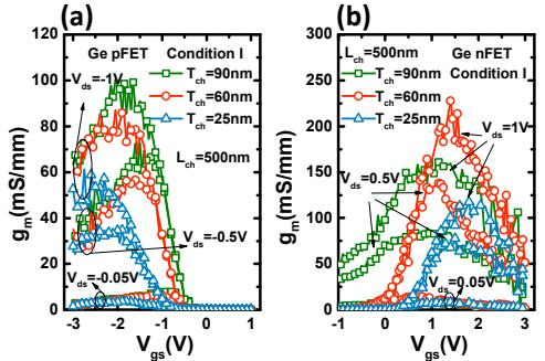
**Fig. 16** (a)  $g_m$  v.s.  $V_{gs}$  curves of pFETs with  $T_{ch}$  of 25, 60 and 90 nm in *condition I*. (b)  $g_m$  v.s.  $V_{gs}$  curves of nFETs with  $T_{ch}$  of 25, 60 and 90 nm in *condition I*.
