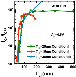
**Fig. 14**  $I_{ON}/I_{OFF}$  ratio scaling metrics of nFETs with  $T_{ch}$  of 15/25 nm in *condition I* and  $T_{ch}$  of 25 nm in *condition III* at  $V_{ds}$  of 0.5 V.
