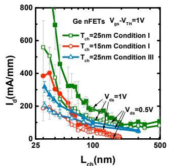
Fig. 11 I<sub>d</sub> scaling metrics of nFETs with T<sub>ch</sub> of 15/25 nm in condition I and T<sub>ch</sub> of 25 nm in condition III at V<sub>gs</sub>-V<sub>TH</sub> = 1V and V<sub>ds</sub> of 0.5 and 1 V.
