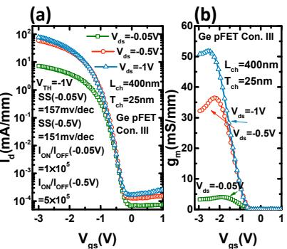
Fig. 7 I<sub>d</sub>-V<sub>gs</sub> curves of a 400 nm L<sub>ch</sub> pFET in condition III with a high I<sub>ON</sub>/I<sub>OFF</sub>. (b) The g<sub>m</sub>-V<sub>gs</sub> curves of the device in (a).
