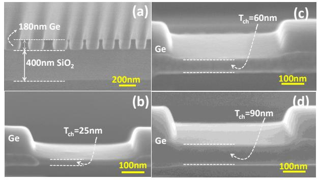
Fig. 3 (a) Cross section of testing recessed channel. A substrate with 180 nm Ge on 400 nm SiO<sub>2</sub> was used. (b-d) Cross sections of recessed channels with T<sub>ch</sub> of 25, 60 and 90 nm, respectively.
