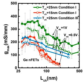
Fig. 12 g<sub>max</sub> scaling metrics of nFETs with T<sub>ch</sub> of 15/25 nm in condition I and T<sub>ch</sub> of 25 nm in condition III at V<sub>ds</sub> of 0.5 and 1 V.
