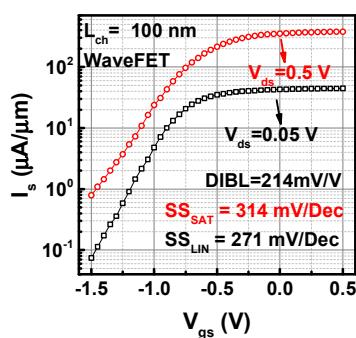
Fig. 14 Transfer characteristics of an InGaAs WaveFET with  $L_{ch}=100\text{nm}$ , 10 nm  $\text{Al}_2\text{O}_3$  as dielectric, where SCEs become severe.
