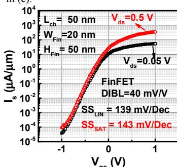
Fig. 10 Transfer characteristics of an InGaAs FinFET with  $L_{ch}=50\text{nm}$ ,  $W_{Fin}=20\text{nm}$ ,  $H_{Fin}=50\text{nm}$  and 10nm Al<sub>2</sub>O<sub>3</sub> as dielectric.
