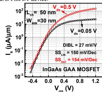
Fig. 12 Transfer characteristics of an InGaAs GAA MOSFET with  $L_{ch}=50\text{nm}$ ,  $W_{NW}=30\text{nm}$  and 10 nm Al<sub>2</sub>O<sub>3</sub> as gate dielectric.
