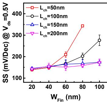
Fig. 16  $W_{Fin}$  dependence of SS at  $V_{ds}=0.5V$  and at various  $L_{ch}$  on InGaAs FinFETs. The InGaAs FinFET devices by wet etching technique show excellent immunity to SCEs down to 50nm with  $W_{Fin}$  less than 40nm, demonstrating nearly vertical sidewall fin structure is critical to be immune to SCEs.
