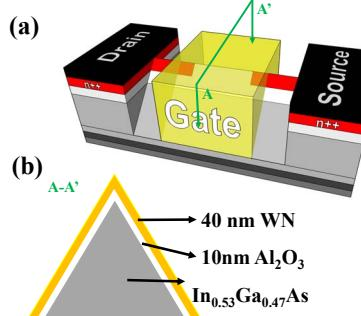
Fig. 2 (a) Schematic diagram and (b) cross-sectional view of an InGaAs MOSFET with a triangle shape. An array of triangles looks like a wave so that we call the device WaveFET.<sup>24</sup>
