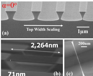
Fig. 7 (b) SEM cross-sectional view of nanowire formation by Ti mask width scaling. An inverted triangular InGaAs structure is formed due to the anisotropic wet etching. (b) The bird eye view and (c) top view of fabricated InGaAs nanowires. InGaAs nanowires can be scaled down to  $W_{NW}=10\text{ nm}$  and  $L_{NW}=1\mu\text{m}$ , as shown in (c).
