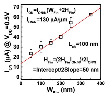
Fig. 15 Extraction of effective Fin height ( $H_{Fin}$ ) by linear fitting of  $I_{ON}$  at  $V_{DD}=0.5V$  versus  $W_{Fin}$ .  $H_{Fin}$  is extracted equals to 50nm determined by the depth of ion implantation. Normalized  $I_{ON}$  at  $V_{DD}=0.5V$  for  $L_{ch}=100\text{nm}$  devices is extracted as  $130\mu\text{A}/\mu\text{m}$ .
