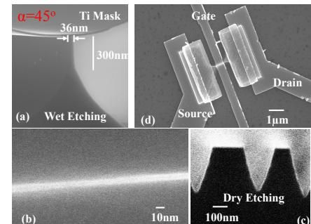
Fig. 9 (a) SEM cross-sectional view of the fin structure. Nearly vertical sidewalls are formed. Fin width is 36 nm and fin height is around 300 nm. (b) The top view of fabricated an InGaAs fin with fin width down to sub-10 nm. (c) InGaAs fins fabricated by Cl-based dry etching where vertical sidewalls are difficult to realize. (d) SEM top view of a fabricated InGaAs FinFET device.
