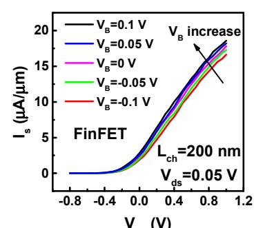
Fig. 21 Body voltage dependence of transfer characteristics at  $V_{ds}=0.05V$  on an InGaAs FinFET with  $L_{ch}=200\text{nm}$ .
