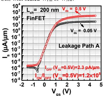
Fig. 22 Transfer characteristics of an InGaAs FinFET on bulk InGaAs with  $L_{ch}=200\text{nm}$  and record  $I_{ON}/I_{OFF}=1.2\times 10^8$ . The high  $I_{ON}/I_{OFF}$  is obtained by barrier engineering on the off-state leakage path.
