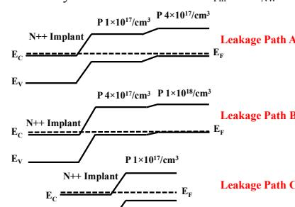
Fig. 23 Summary of energy barriers for possible off-state leakage paths of devices in this work. Leakage Path A is for InGaAs FinFET devices fabricated on substrate A. Leakage Path B is for InGaAs FinFET devices fabricated on substrate B. Leakage Path C is for InGaAs devices fabricated on substrate A but without mesa isolation.
