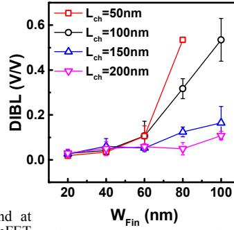
Fig. 17  $W_{Fin}$  dependence of DIBL at various  $L_{ch}$  of InGaAs FinFETs.
