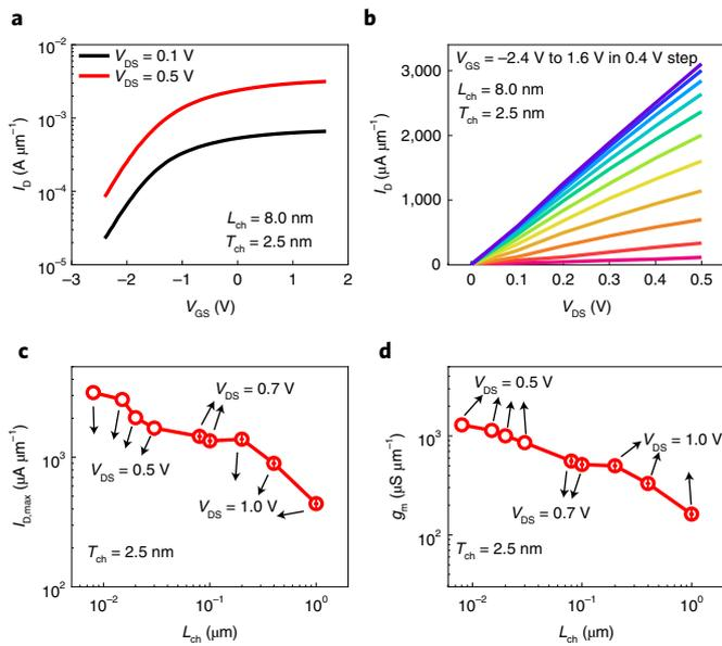
**Fig. 4 | Channel length scaling of ALD  $\text{In}_2\text{O}_3$  transistors down to 8 nm.**
