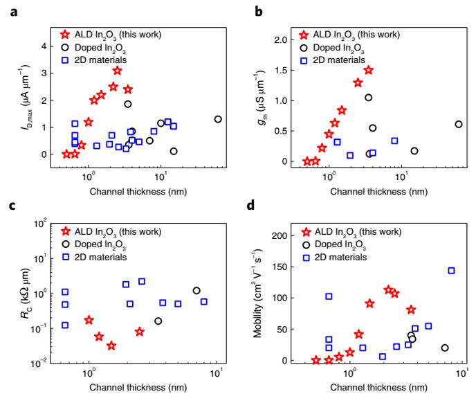
**Fig. 5 | Benchmarking of ALD  $\text{In}_2\text{O}_3$  with other ultrathin semiconductors.**
