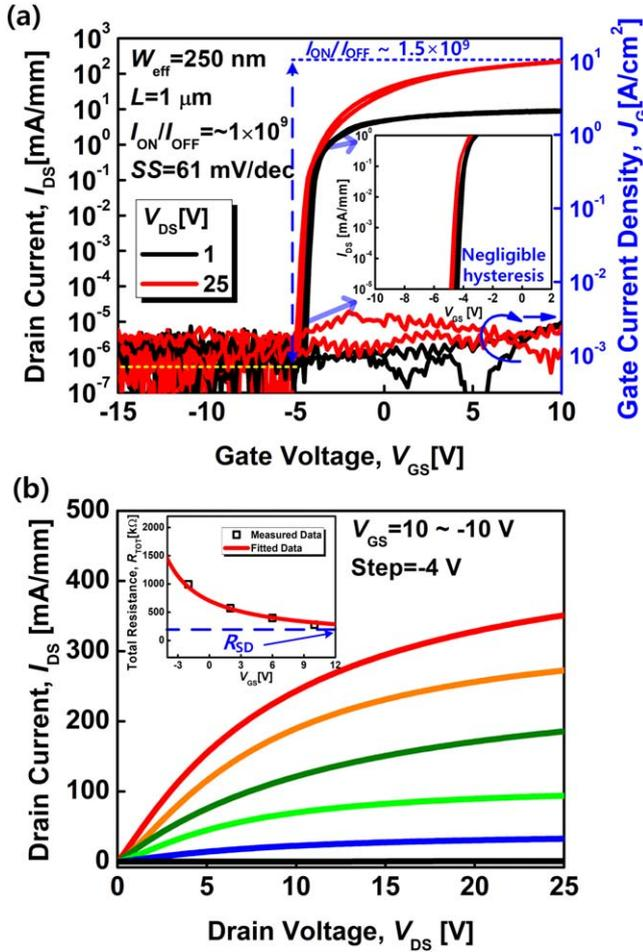
**Figure 2.** (a) Measured  $I_{DS}$ - $V_{GS}$  transfer characteristics and (b)  $I_{DS}$ - $V_{DS}$  output characteristics of the fabricated tri-gate  $\beta$ -Ga<sub>2</sub>O<sub>3</sub> FET.
