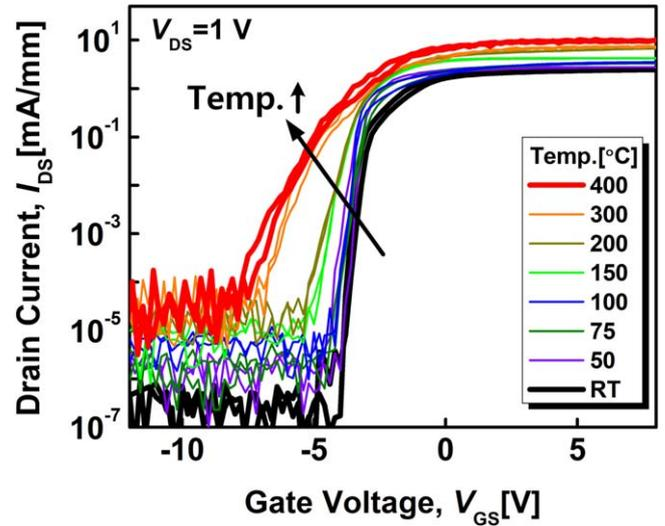
**Figure 3.** Measured  $I_{DS}$ - $V_{GS}$  characteristics of the fabricated tri-gate  $\beta$ -Ga<sub>2</sub>O<sub>3</sub> FETs on SiO<sub>2</sub>/Si substrate at various temperatures ranging from RT to 400 °C.
