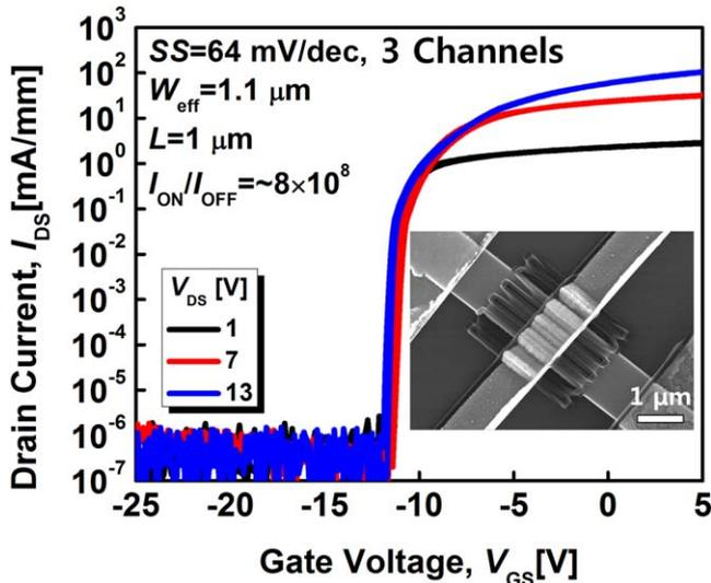
**Figure 5.** Measured  $I_{DS}$ – $V_{GS}$  characteristics of the fabricated  $\beta$ -Ga<sub>2</sub>O<sub>3</sub> FETs with multi-channels. Inset shows SEM image for top view of the fabricated device with 3 channels.
