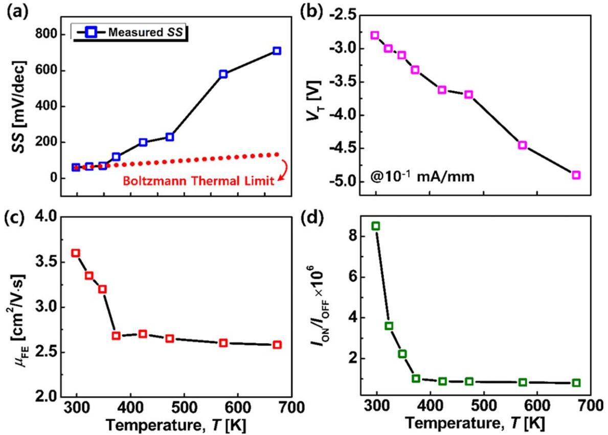
**Figure 4.** Temperature dependences (RT–400 °C) at  $V_{DS} = 1$  V of typical device parameters such as (a) SS (dashed line: Boltzmann thermal limit of SS), (b)  $V_T$ , (c)  $\mu_{FE}$ , and (d)  $I_{ON}/I_{OFF}$  of the tri-gate  $\beta$ -Ga<sub>2</sub>O<sub>3</sub> FETs on the SiO<sub>2</sub>/Si substrate.
