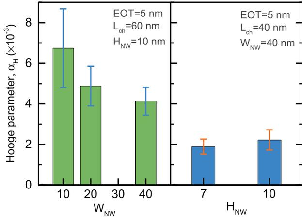
Fig. 6. Hooge parameters in Ge NW nMOSFETs with (a)  $W_{NW}$  of 10, 20, 30, and 40 nm and (b)  $H_{NW}$  of 7 and 10 nm.
