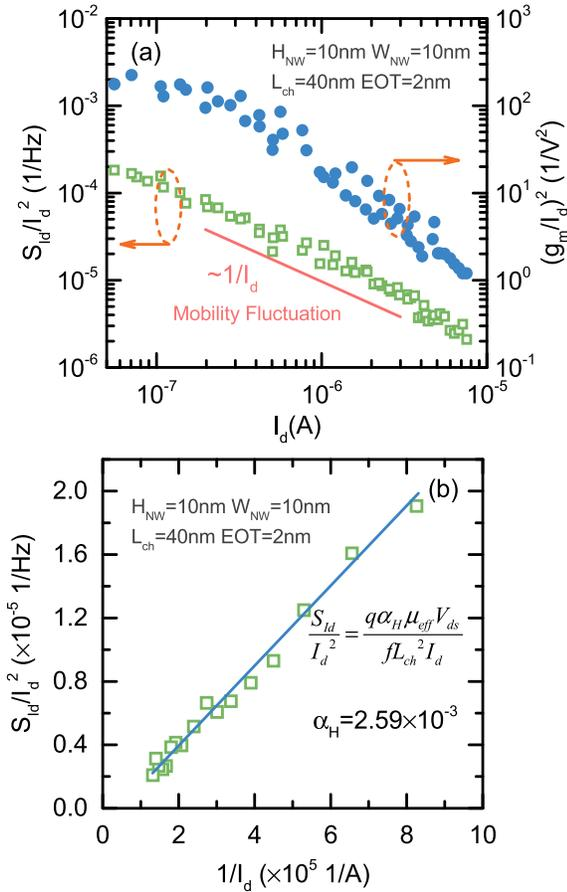
Fig. 3. (a) Normalized  $S_{Id}$  and  $(g_m/I_d)^2$  versus  $I_d$  of devices with  $1/f$  low-frequency noise at 10 Hz. (b)  $S_{Id}/I_d^2$  versus  $1/I_d$  at 10 Hz and the linear fit. The Hooe parameter is  $2.59 \times 10^{-3}$ .
