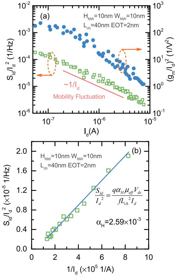
Fig. 3. (a) Normalized  $S_{Id}$  and  $(g_m/I_d)^2$  versus  $I_d$  of devices with  $1/f$  low-frequency noise at 10 Hz. (b)  $S_{Id}/I_d^2$  versus  $1/I_d$  at 10 Hz and the linear fit. The Hooge parameter is  $2.59 \times 10^{-3}$ .
