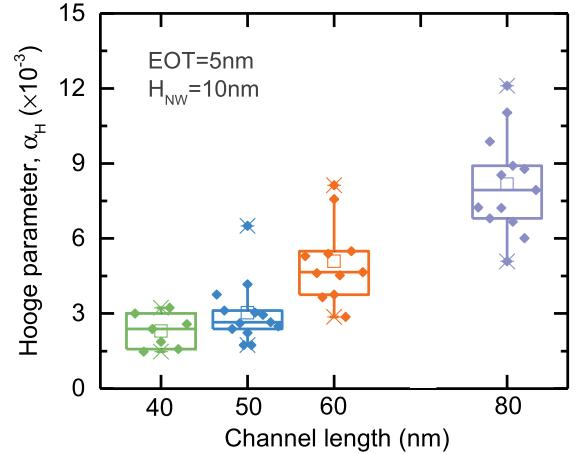
Fig. 5. Box plot of the Hooge parameters of devices with a channel length from 40 to 80 nm. The Hooge parameter decreases with the scaling down of  $L_{ch}$ .
