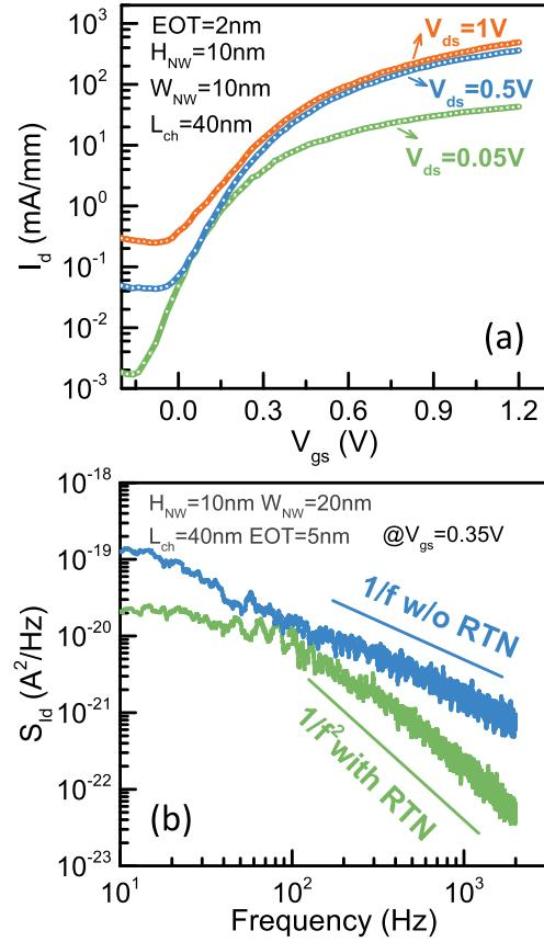
**Fig. 2.** (a) Transfer characteristics of a 40-nm  $L_{\text{ch}}$  NW nMOSFET. (b)  $S_{\text{Id}}$  of two devices, having the same device dimensions, with and without RTNs at  $V_{\text{gs}}$  of 0.35 V.
